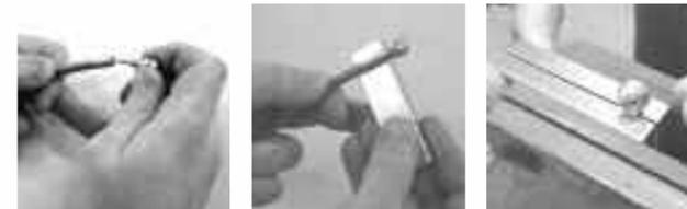
Push a small bradawl into the hose to make the tube as round as possible. Push the hose tail into the centre of the ferrule until it is fully in.
