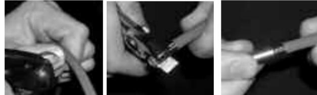
Cut hose to required length using cutters supplied.
