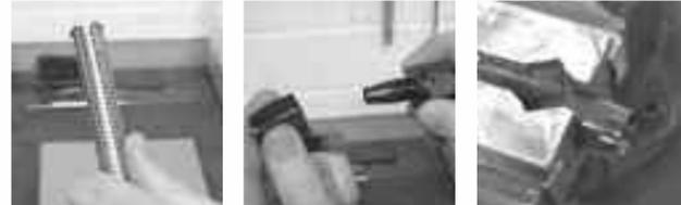
Cut hose to required length using suitable fine tooth hacksaw or cut off machine. Remove any debris from inside the hose.
