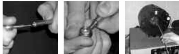
Locate the tip of the fitting just inside the teflon tube and push fitting into the hose.
