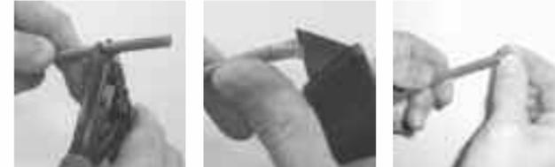
Cut hose to suit your system using sharp cable cutters or a small hacksaw. This pvc cover comes off easily without force blade.
